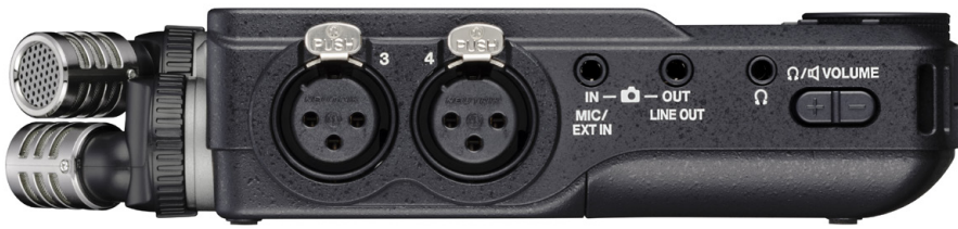
■ The Portacapture X6 can capture two external mics, with the XLRs capable of delivering phantom power and the stereo mini-jack input capable of plug-in power.
