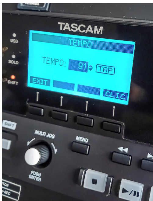
With a push-turn encoder and five buttons, the simple on-screen menus are mercifully quick and easy to navigate.
