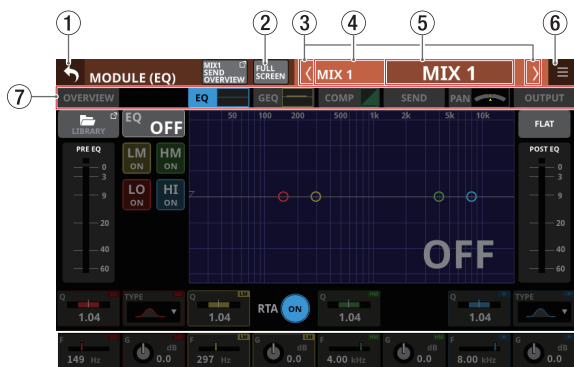
MODULE (EQ) Screen for MIX 1–22 modules
