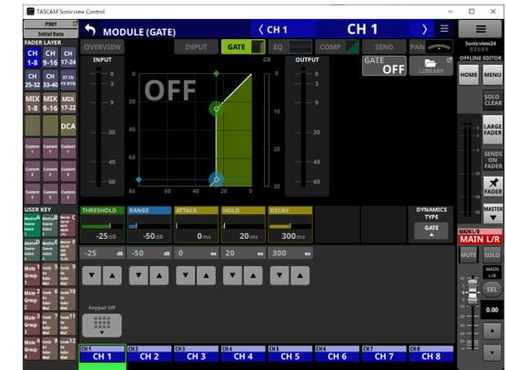
Doing this will replace the Channel Section (⑤) with the Keypad.
