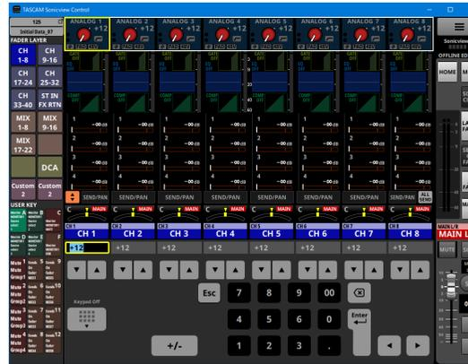
Doing this will replace the Channel Section (⑤) with the Keypad.
